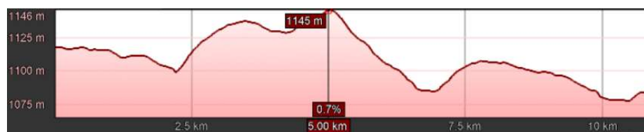
Figure 5-28: Elevation profile of the Water pipe line for distribution lines of Nyakabale RGC
