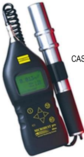
Photo 4-1: Digital CASELLA microdust and 6-gas MX6 iBrid™ meters to be used to measure air quality
