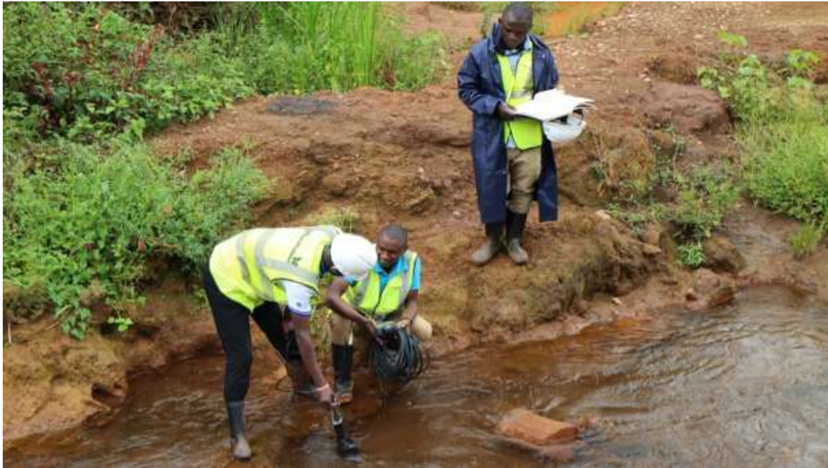
Figure 3-10: In situ water quality measurements using Horiba U-53 water quality meter along Mishumba at E232809, N9903119.
