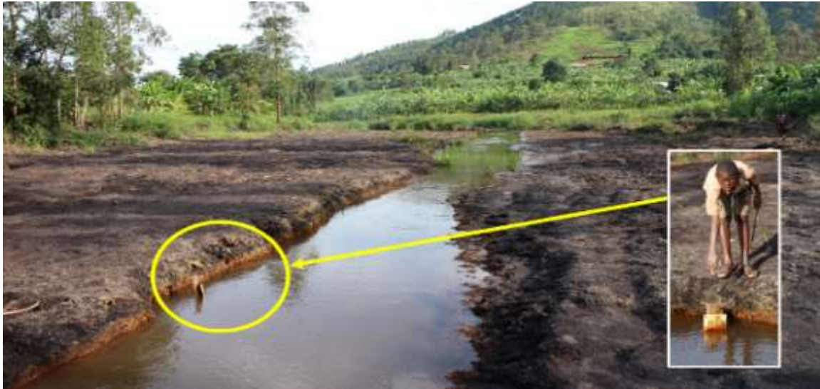
Figure 4-10: Temporary gauging station along R. Mishumba (36 M E 232879, N 9899582) downstream of the dam site and its current status
