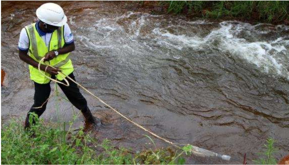
Figure 3-7: Zooplankton sampling from the mid water column using a conical net
