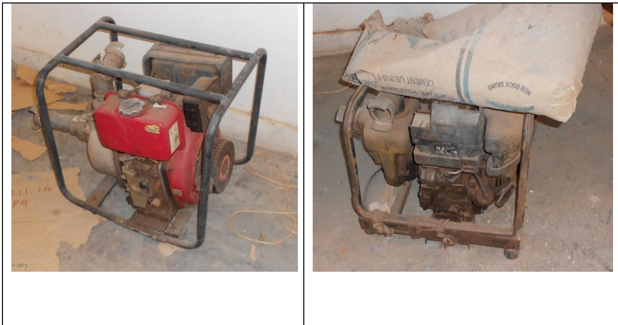
Figure 1-10: Raw water pumps for the mini piped water supply scheme
