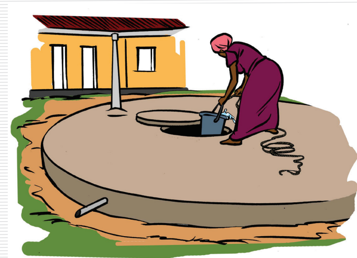
Figure 29: Completed underground tank with a bucket for drawing water
