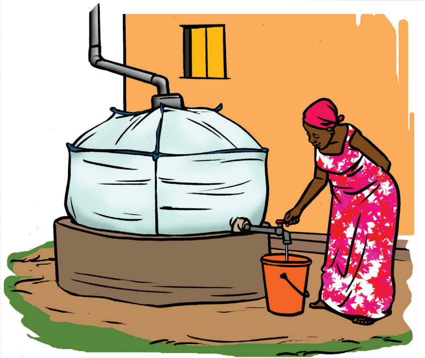
Figure 49: Install the gutters and tap
