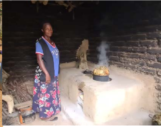
Photo3-9 Improved household Sove (Rocket Lorena Stove) at a beneficiary's homestead in Masaka District
