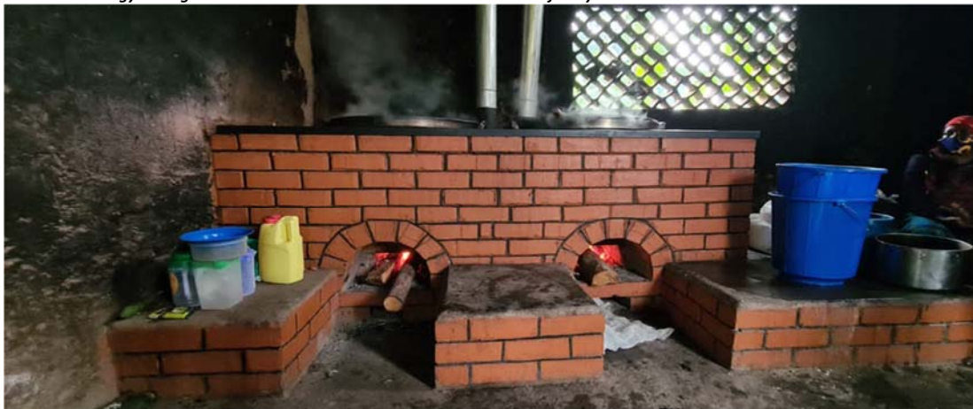
Photo 3-10: Institutional Energy Saving Stove at Kijabwemi Church of Uganda (CoU) Primary School in Masaka District
