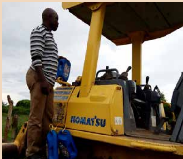
Changing engine oil of a Komatsu Bull dozer
