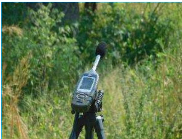
Casella CEL-633B noise meter on a tripod stand (1.2m high) from the ground
