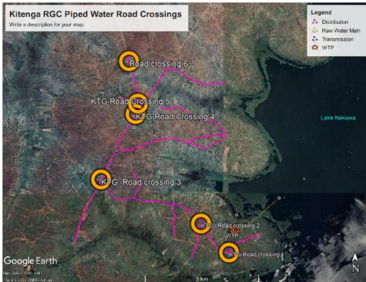
Figure 2-13: Major pipeline access road crossing
