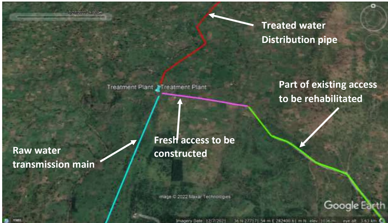
Figure 2: Access to the Nyagak Water Treatment Plant
