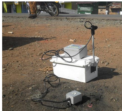
Photo 14: Vibration measurement meter (Nomis SuperMini® Seismograph)
