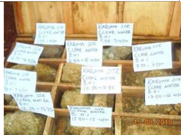
Plate 17.0: Clear Water Tank Samples
