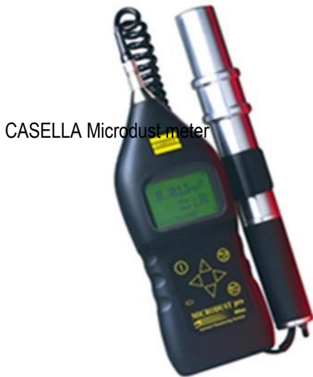
Photo 12: Digital CASELLA microdust and 6-gas MX6 iBrid™ meters to be used to measure air quality
