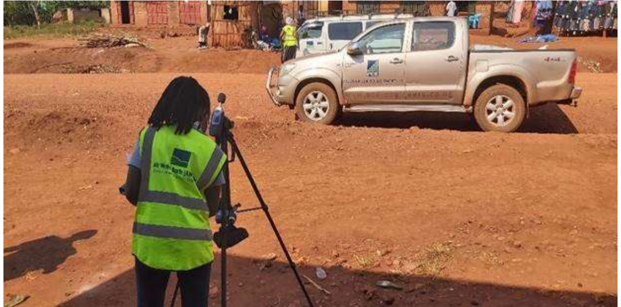
Photo 5-3 Ambient Air quality and Noise level measurements at Bugomolwa Central Trading centre
