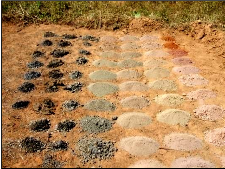
Figure 10: Samples are laid out and logged for 1m depth intervals
