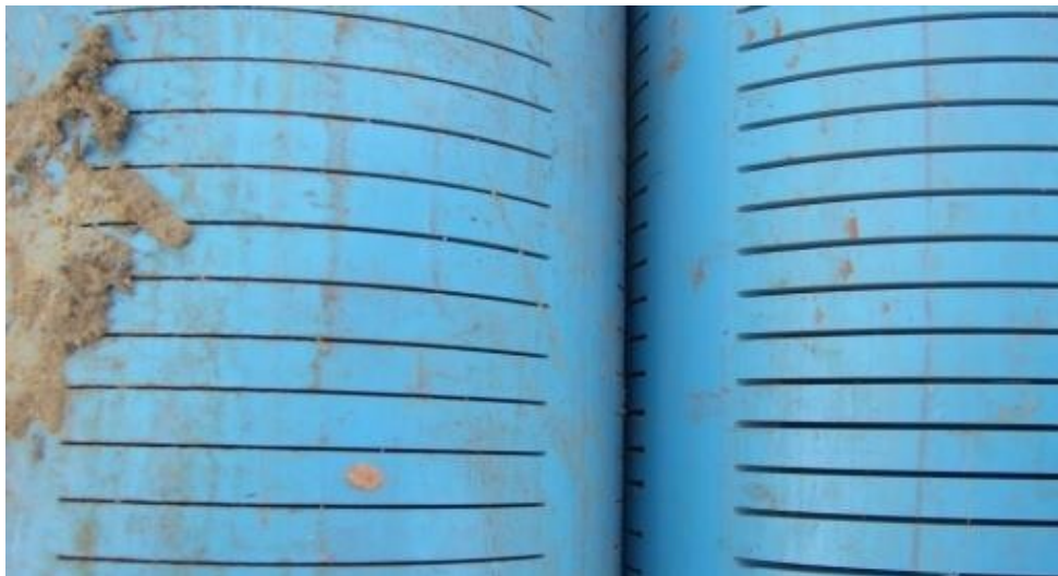
Figure 8: PVC screen slot sizes (left 0.75mm slot, right 1mm slot)
