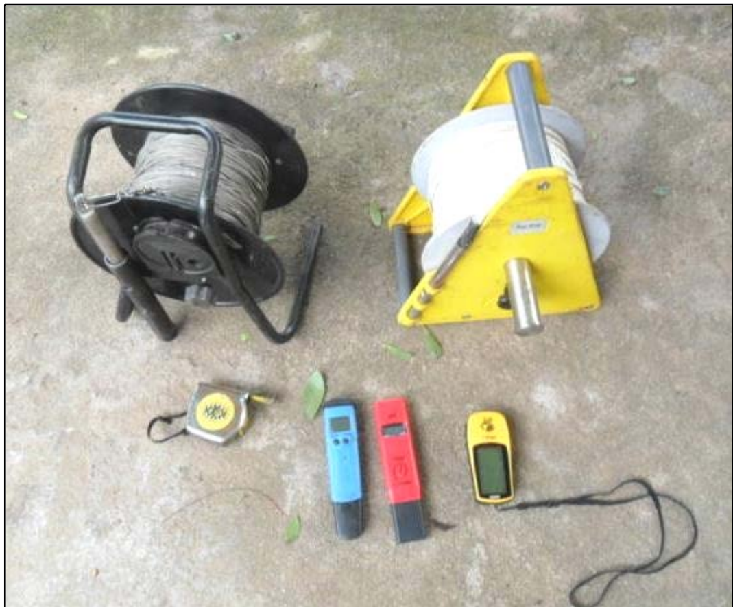
Figure 7: Some common kit items – Depth meter, Electronic dipper, Tape, EC and PH meters, Handheld Global Positioning System (GPS) device
