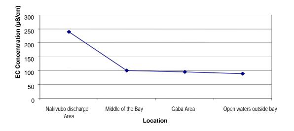
FIG. 3. Inner Murchison Bay mean electrical conductivity (EC) profile from discharge point to open waters.
