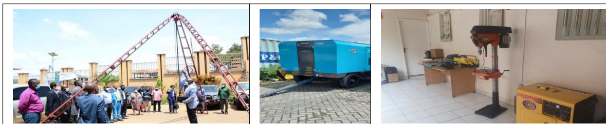
Inset is some of the specialised equipment provided by JICA to the regional service support and rehabilitation centre in Mubende for specialised support. This includes Tripod stand with chain block for major repair of borehole (Extreme left), Air lifting compressors for water well cleaning (Centre) and workshop equipment (Extreme Right) to start up the repair workshop in Mubende
