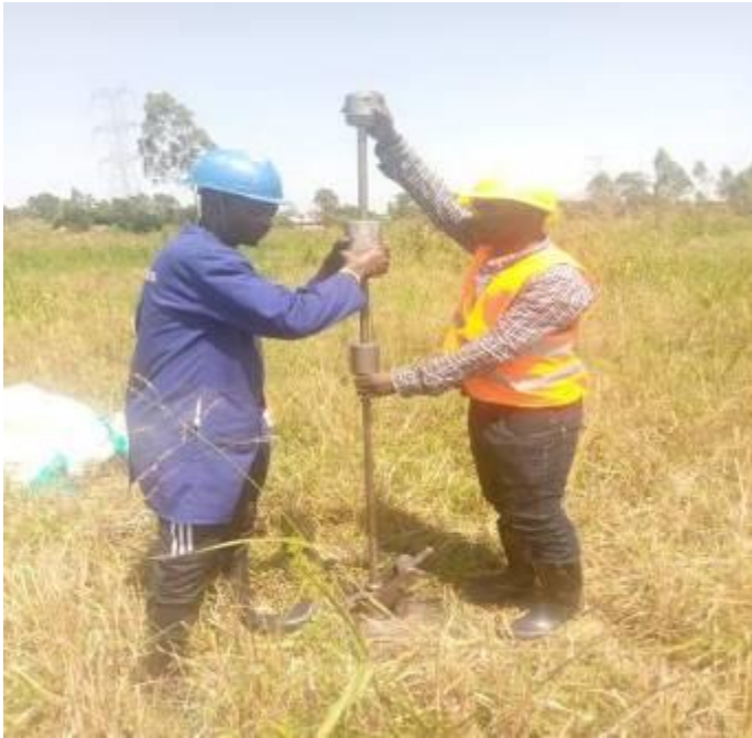
Figure 2-2: Conducting of the DPL test at site
