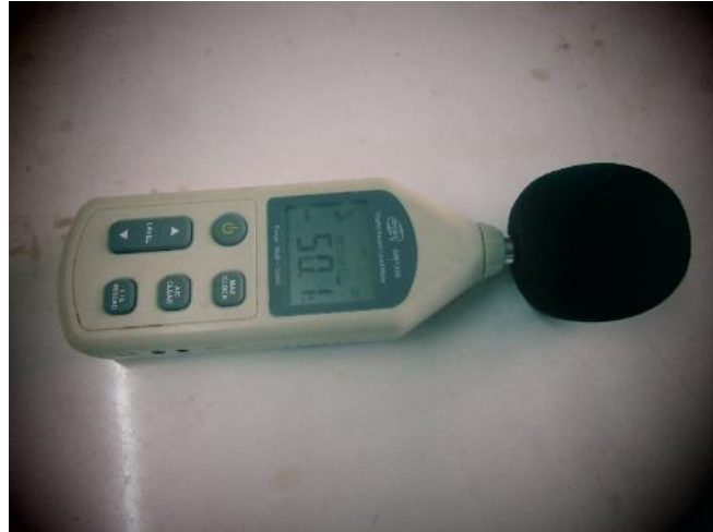
Plate 2: Noise level meter used for noise assessment. Taken by the Environmentalist, March 2023
