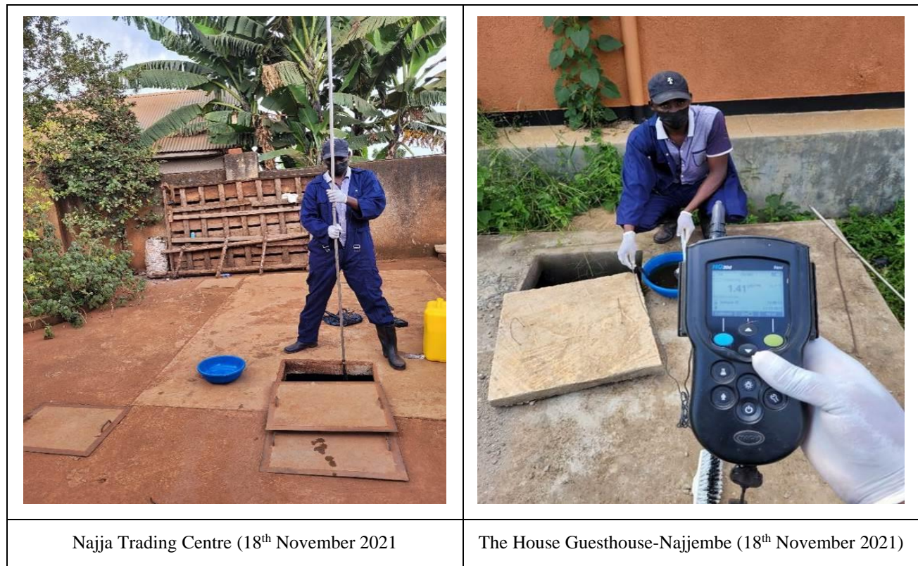
Figure 2-1: Faecal sludge sampling onsite sanitation facilities using a sampler
